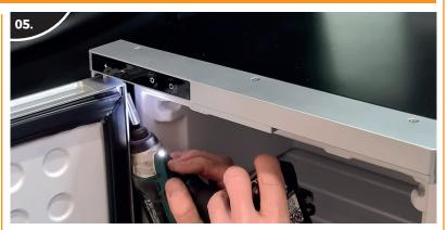
Now Refit the Top display panel by screwing the 3 top screws in and then the hinge screw underneath.
