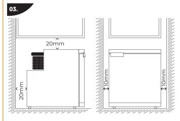
Before fitting, line the unit up and dummy fit to the space for the appliance. Remember to leave specified gaps to ensure cold temperature efficiency.
