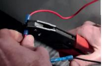
Then the connection should be crimped, use a heat gun to shrink the connector to the wiring.
